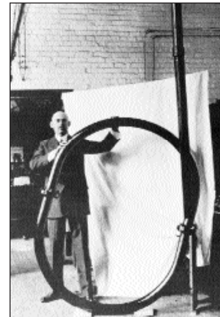
Circular tube used in proving further that a rocket would provide thrust in a vacuum, 1915.
