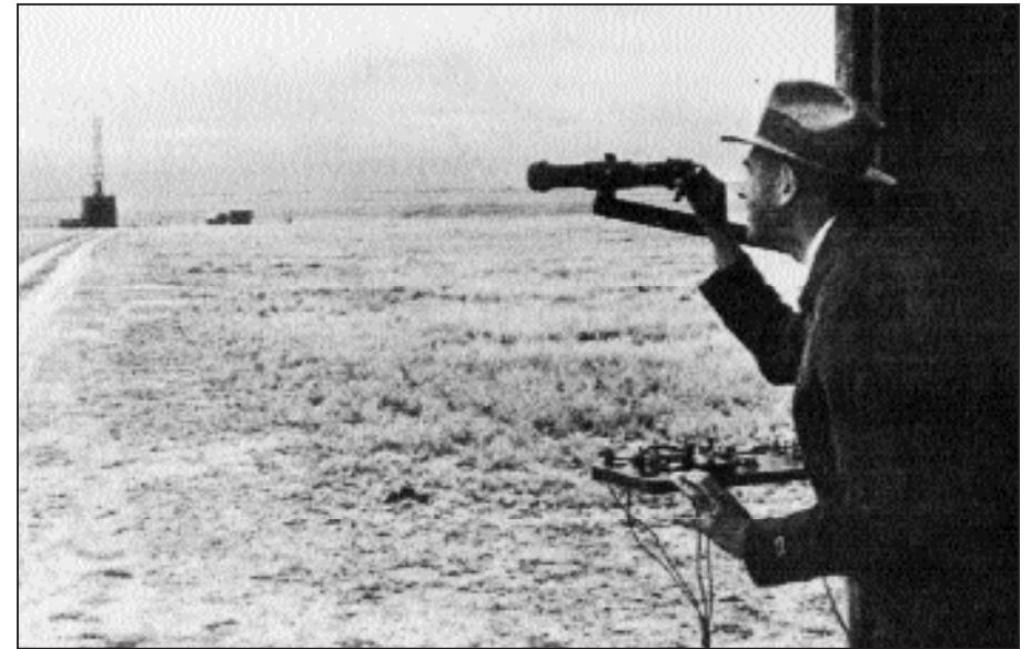
Goddard at his launch command post, Eden Valley, late 1930s. The telescope focused on gauges connected to pressure lines on the rocket in the launch tower. When readings were right, he could operate fire, release, or stop keys on the panel in front of him.
