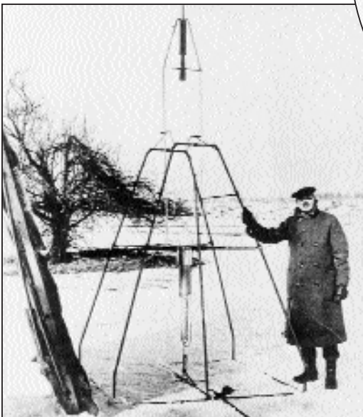
Goddard posing with the rocket in its launch frame, shortly before the first liquid-fuel rocket flight, "Aunt Effie" Ward's farm, Auburn, Massachusetts, 16 March 1926. This is the most familiar photo of Goddard ever taken, distributed by the photographer, his wife Esther, in the decades after his death.
